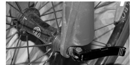
An improperly closed quick-release.
