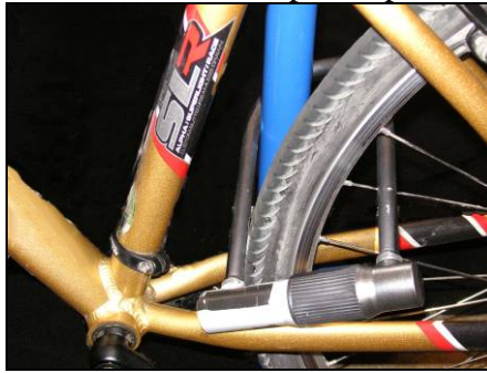
The frame is automatically secured if the rear wheel is locked inside the rear triangle.
